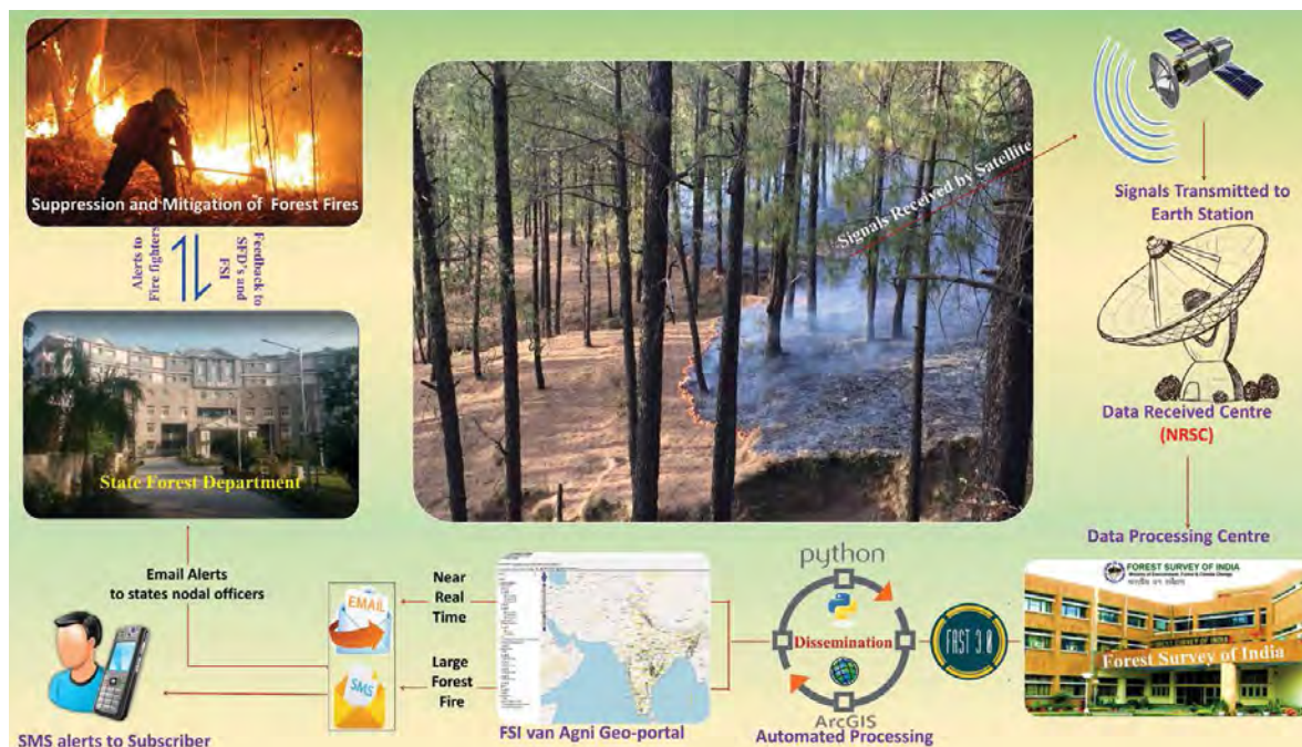
FIGURE 5.1 Work flow of near real time forest fire monitoring
