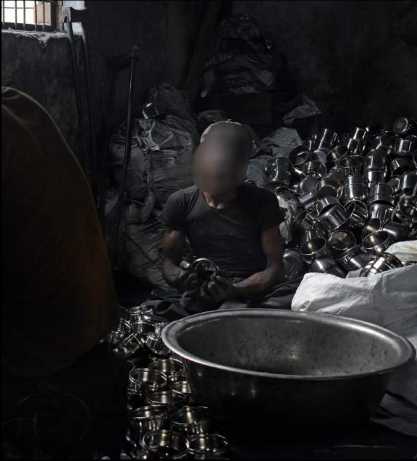
A worker doing the final polish.
